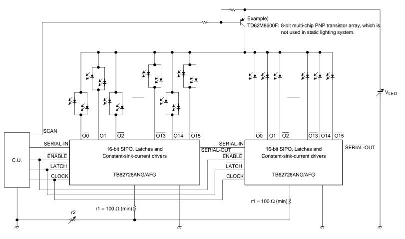
Application Circuit (example 2): When the condition of VLED is VLED > 17 V
