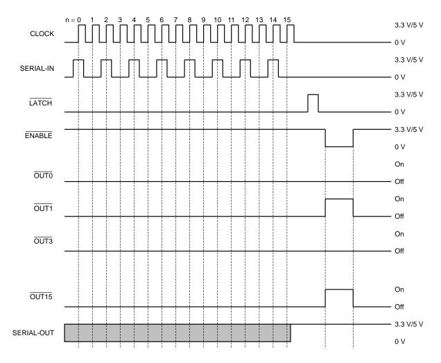
Warning: Latch circuit is leveled-latch circuit. Be careful because it is not triggered-latch circuit.
