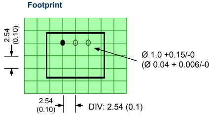
Dimensions are typical values: mm (inch) General Tolerance:  $\pm 0.25 (\pm 0.01)$ Pin Tolerance:  $\pm 0.1 (\pm 0.004)$
