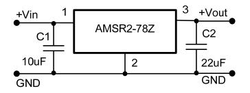
C1: A low ESR capacitor is required to keep the noise of the converter to a minimum. Ceramic capacitors are recommended with typical value is  $10\mu$ F / 25V.
