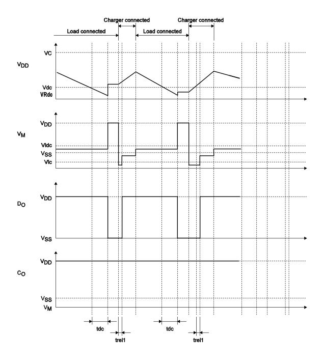
VC : Over-charge detection voltage tdc : Over-discharge detection delay time
