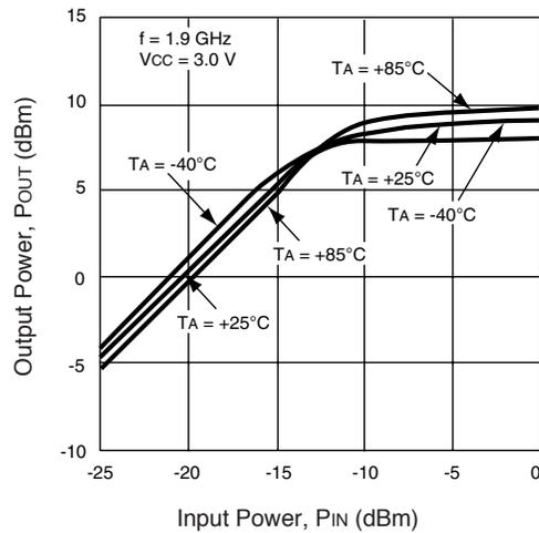
**SATURATED OUTPUT POWER vs. FREQUENCY AND VOLTAGE**
