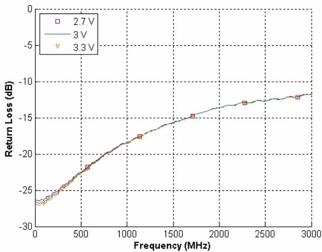
**Figure 14. Return Loss: RF1/RF2 @ 3.0 V**
