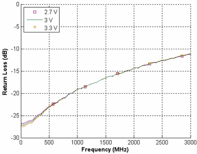
Figure 16. Return Loss: RFC/RF1 @ 3.0 V
