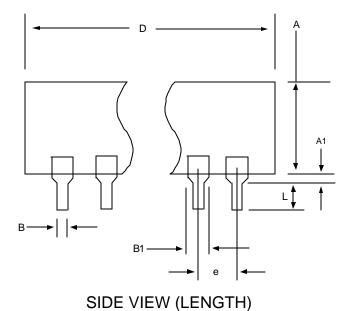
Package Dimensions for 40 Lead PDIP (600 mil.)
