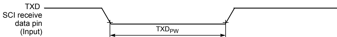
Figure 10-16 TXD Pulse Width
