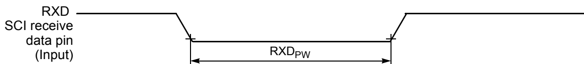
Figure 10-15 RXD Pulse Width
