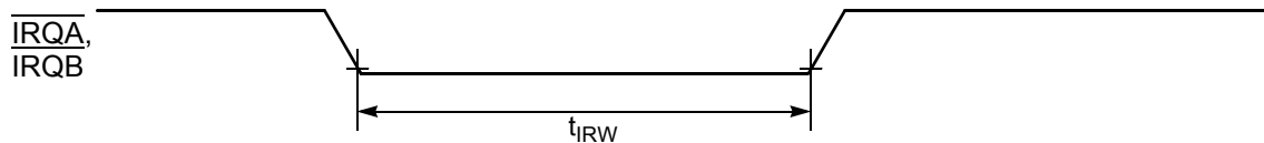
Figure 10-5 External Interrupt Timing (Negative Edge-Sensitive)
