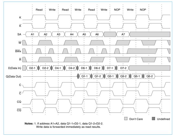
Read, Write, and NOP Timing Diagram
