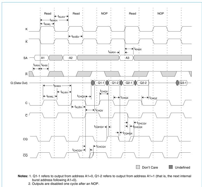
**Read and Deselect Cycles Timing Diagram**
