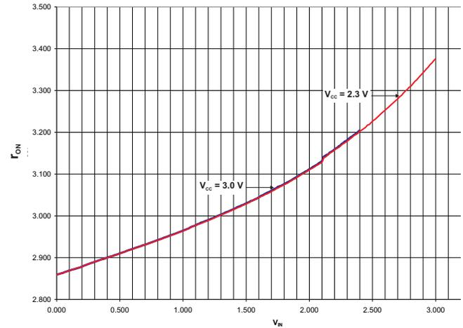
Figure 4.  $r_{ON}$  ( $I_{OUT} = -15$  mA)
