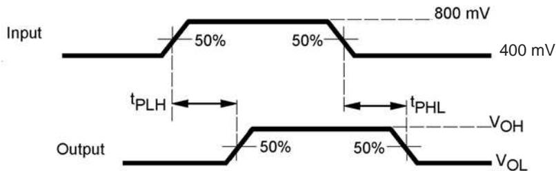
Figure 10. Propagation Delay
