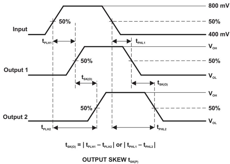
Figure 11. Skew Test
