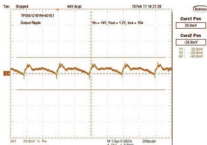
Figure 23. Output Ripple 20 mV/div, 1.0 μs/div, 20 MHz Bandwidth, AC Coupled
