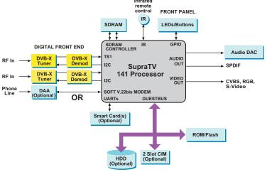
For cable set-top boxes use DVB-C tuner & QAM demodulator
