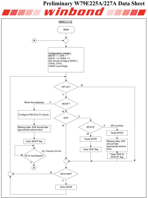
Figure 18-13: SPI multi-master slave s/w flow diagram
