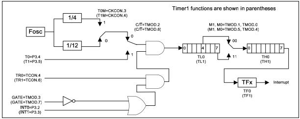
Figure 12-1: Timer/Counters 0 & 1 in Mode 0 and Mode 1
