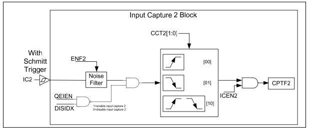
Figure 15-3: Input Capture 2 block diagram
