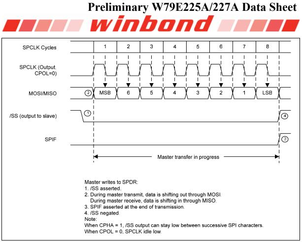
Figure 18-4: Master Mode Transmission (CPOL = 0, CPHA = 1)
