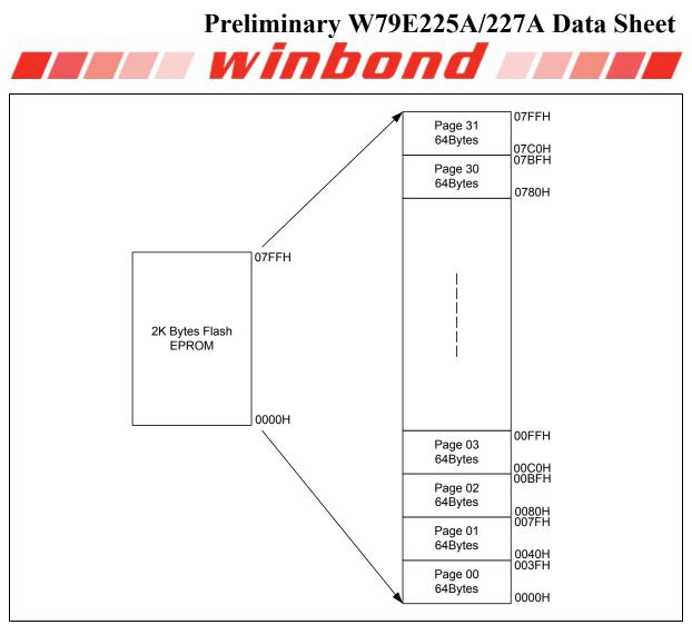
Figure 6-3: W79E227 NVM Memory Mapping
