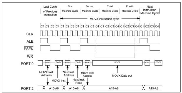
Figure 8-8: Data Memory Write with Stretch Value = 2
