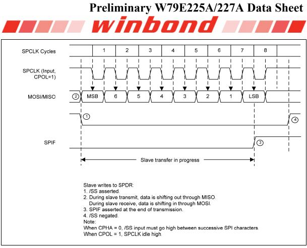
Figure 18-7: Slave Mode Transmission (CPOL = 1, CPHA = 0)
