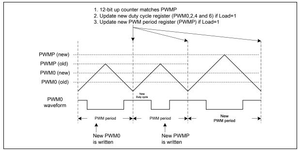
Figure 14-20: Center-Aligned Mode
