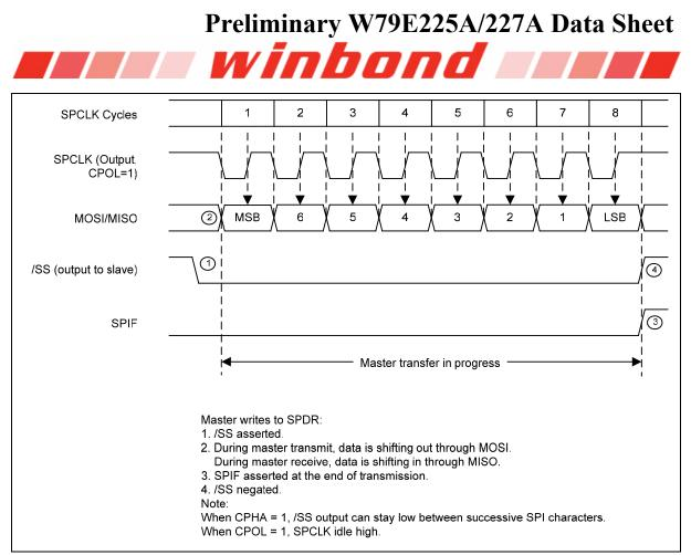
Figure 18-5: Master Mode Transmission (CPOL = 1, CPHA = 1)
