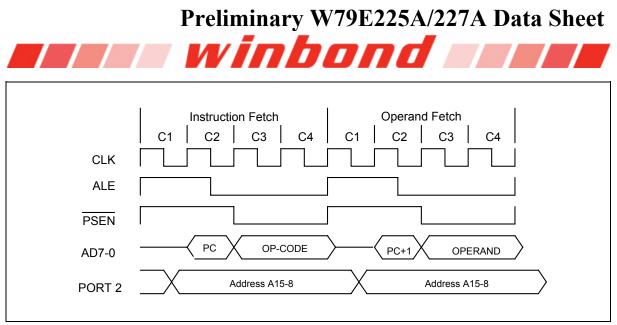
Figure 8-2: Two Cycles Instruction Timing
