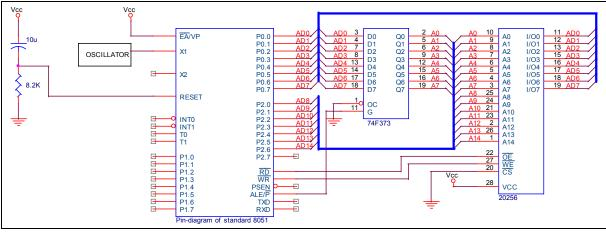
Figure 25-2: Typical External Data Memory and Oscillator connections
