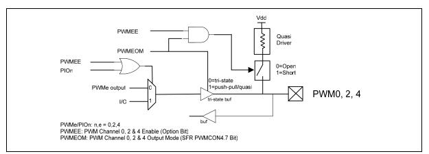
Figure 14-3: PWM0, 2 & 4 I/O pins
