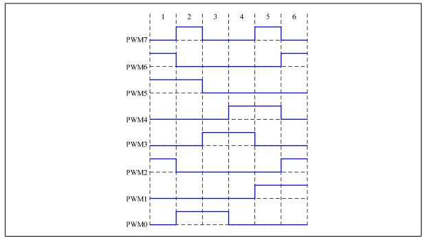
Figure 14-14: Example 1 of Output Even & Odd Override
