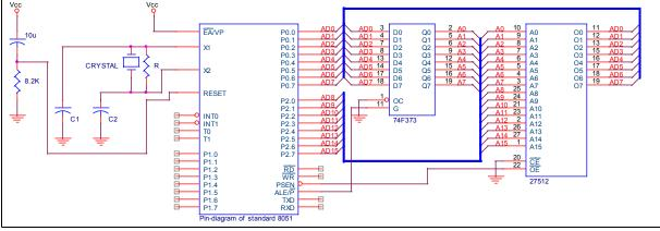
Figure 25-1: Typical External Program Memory and Crystal connections
