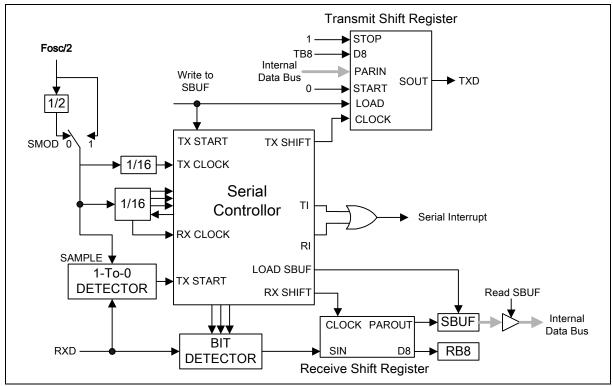
Figure 16-3 Serial Port Mode 2
