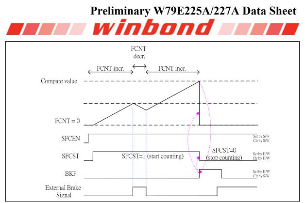
Figure 14-26: Smart Fault Detector timing diagram
