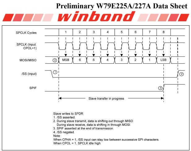
Figure 18-9: Slave Mode Transmission (CPOL = 1, CPHA = 1)
