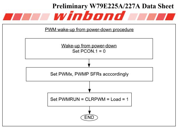
Figure 14-28: Example of PWM wake-up from power-down procedure
