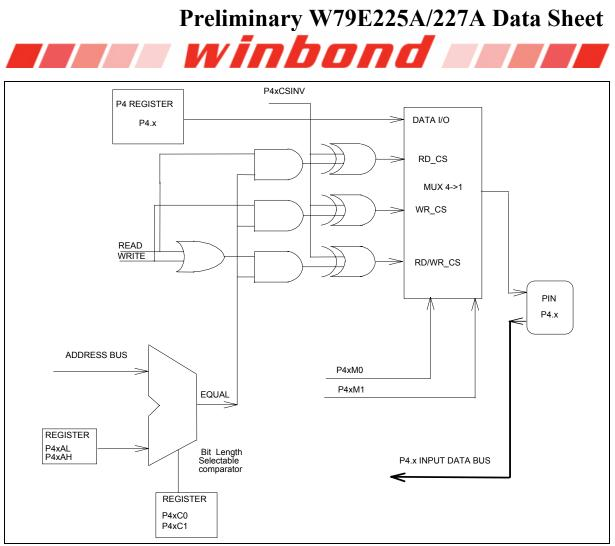
Figure 21-1 Port 4 Structure Diagram
