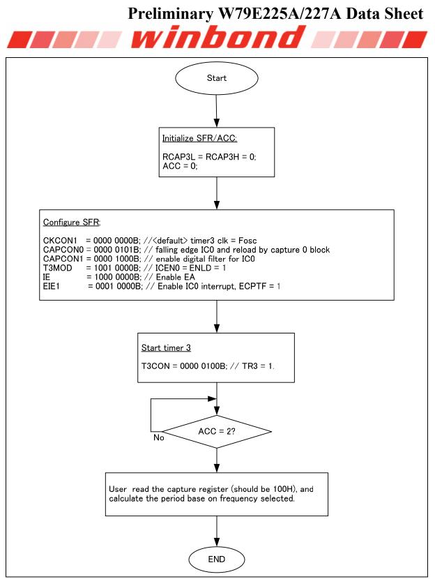
Figure 15-5: Program flow for measurement with IC0 between pulses with falling edge detection (ACC is incremented in interrupt service routine).
