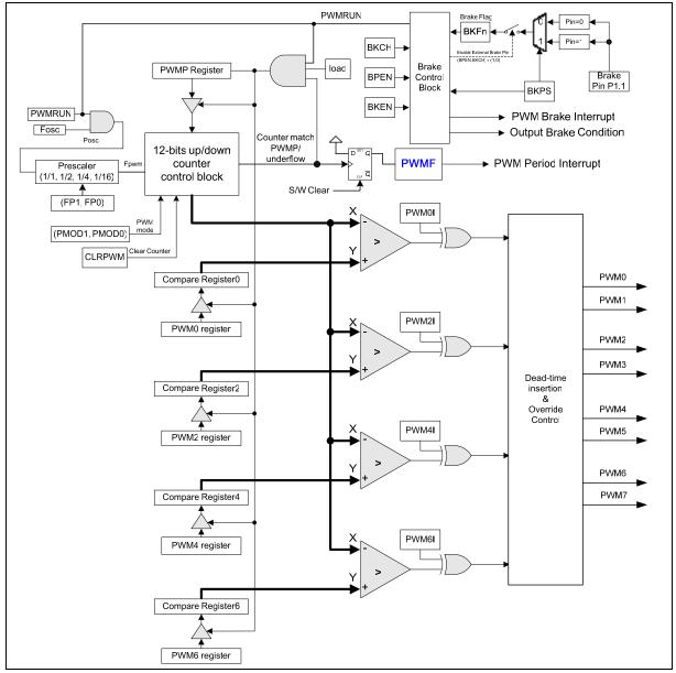
Figure 14-2: PWM Time-base Generator and Brake Function
