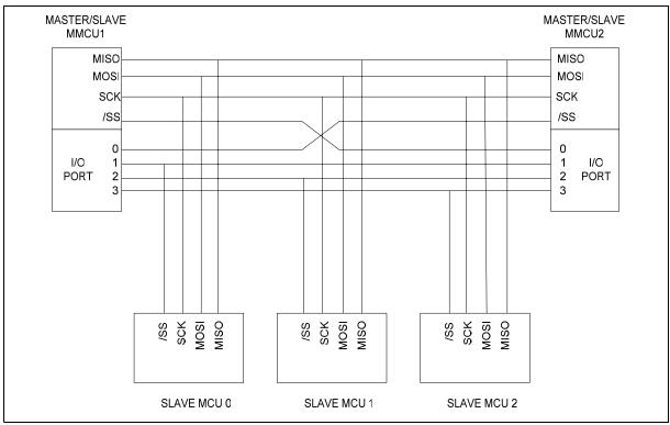
Figure 18-12: SPI multi-master slave environment
