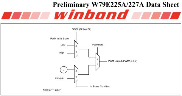
Figure 14-8: Odd PWM Output
