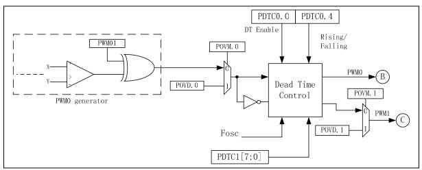
Figure 14-9: Complementary PWM with Dead-time and Override functions
