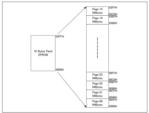
Figure 6-2: W79E225 NVM Memory Mapping
