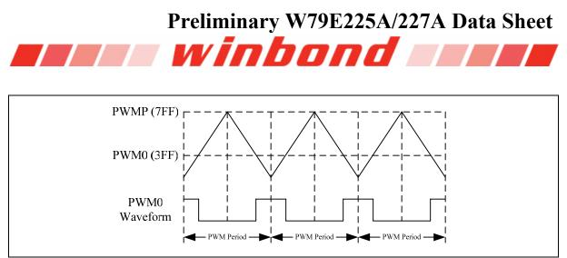
Figure 14-22: PWM0 Center Aligned Waveform Output
