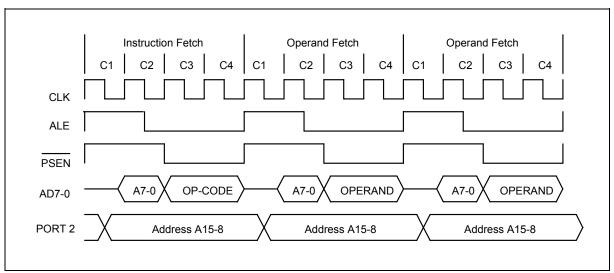
Figure 8-3: Three Cycles Instruction Timing
