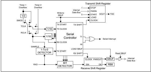
Figure 16-2 Serial Port Mode 1
