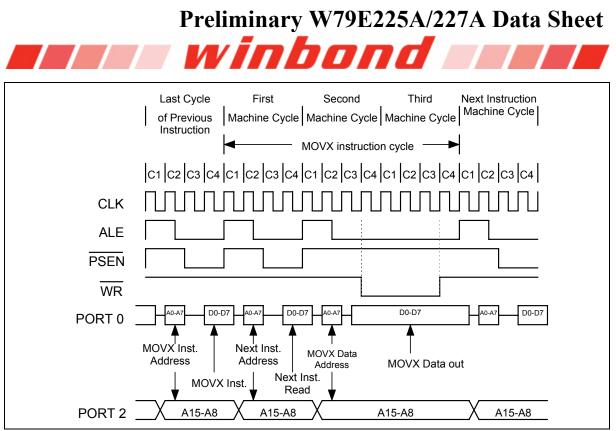
Figure 8-7: Data Memory Write with Stretch Value = 1
