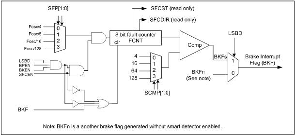
Figure 14-25: Smart Fault Detector
