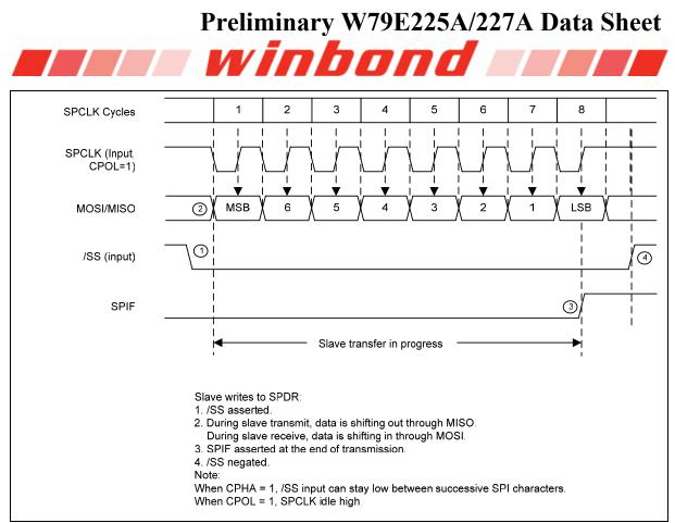
Figure 18-9 show the SPI transfer format, with different CPOL and CPHA. When CPHA = 0, data is sample on the first edge of SPCLK and when CPHA = 1 data is sample on the second edge of the SPCLK. Prior to changing CPOL setting, SPE must be disabled first.
