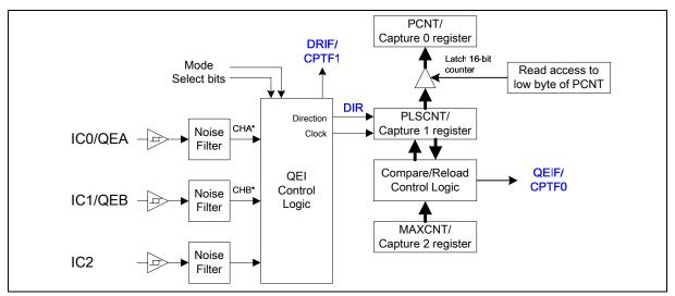
Figure 15-10: QEI Block Diagram
