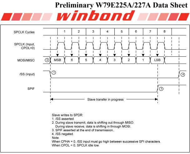
Figure 18-6: Slave Mode Transmission (CPOL = 0, CPHA = 0)
