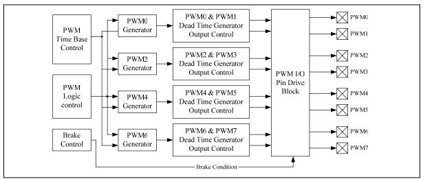
Figure 14-1: PWM Block Diagram
