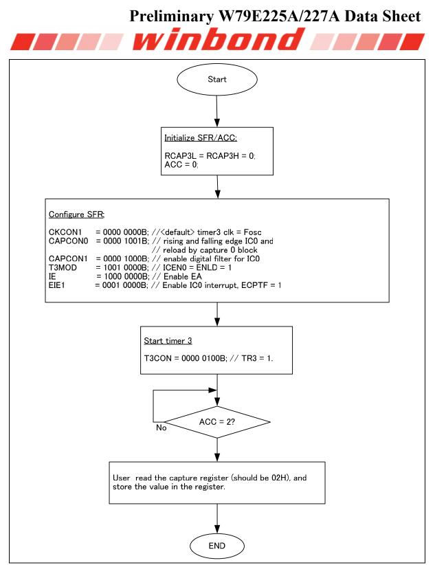
Figure 15-7: Program flow for measurement with IC0 pulse width with rising and falling edge detection (ACC is incremented in interrupt service routine).
