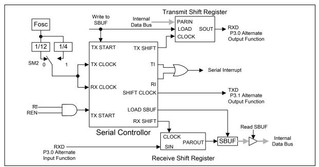
Figure 16-1 Serial Port Mode 0
