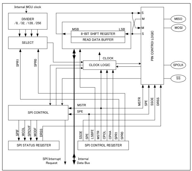
Figure 18-1: SPI block diagram
