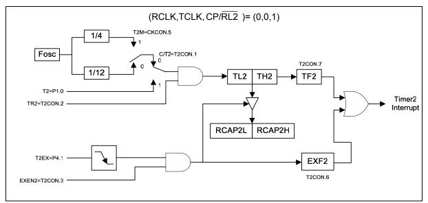
Figure 12-4: Timer2 16-Bit Capture Mode
