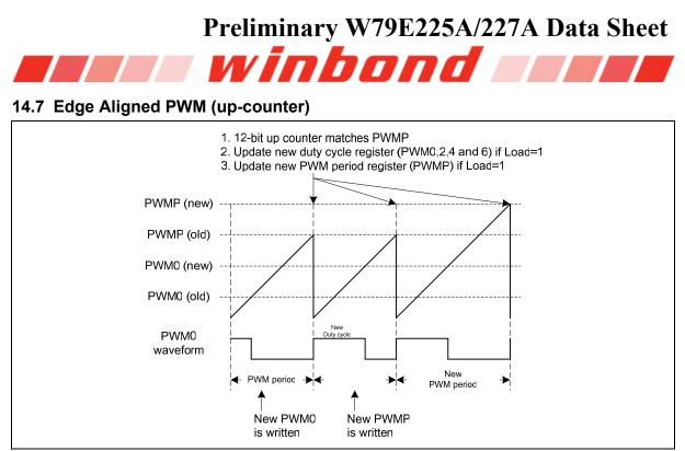
Figure 14-16: Edge-Aligned PWM
