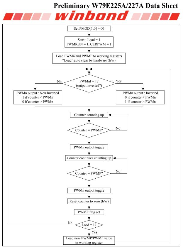
Figure 14-17: Edge-Aligned Flow Diagram
