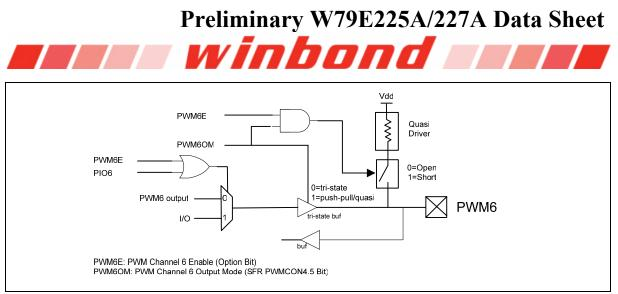
Figure 14-5: PWM6 I/O pin
