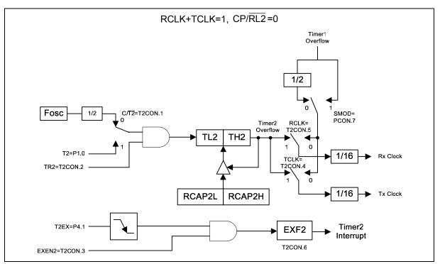
Figure 12-7: Baud Rate Generator Mode
