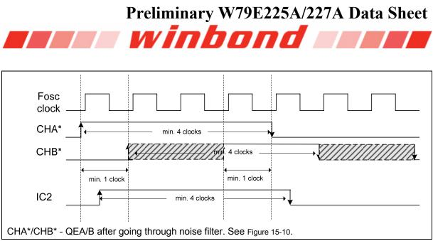
Figure 15-11: QEA/QEB/IC2 timing requirement.
