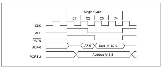
Figure 8-1: Single Cycle Instruction Timing
