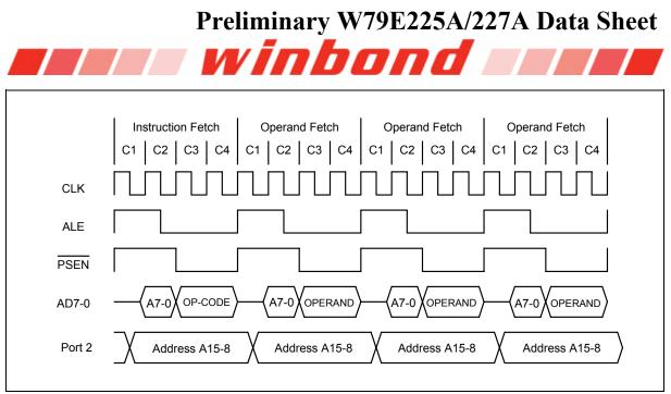
Figure 8-4: Four Cycles Instruction Timing
