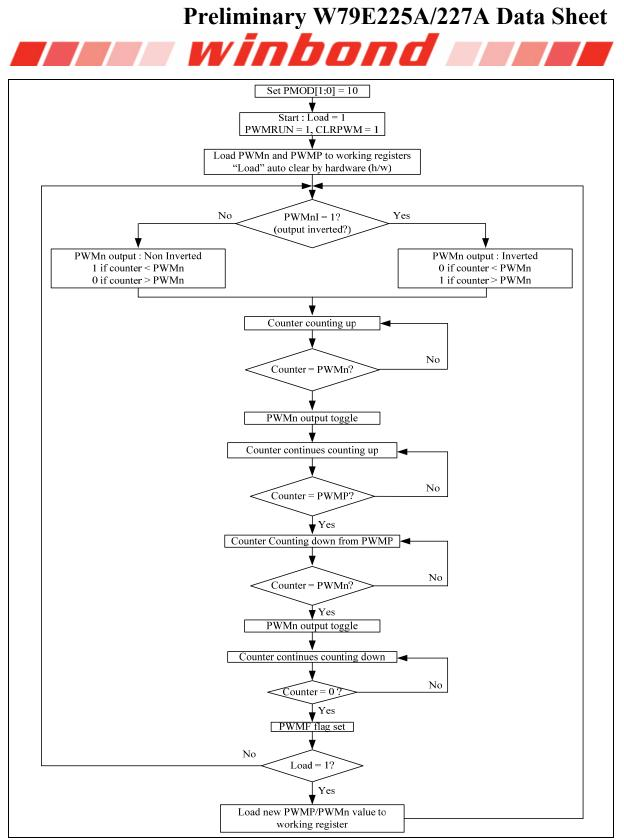
Figure 14-21: Center-aligned Flow Diagram
