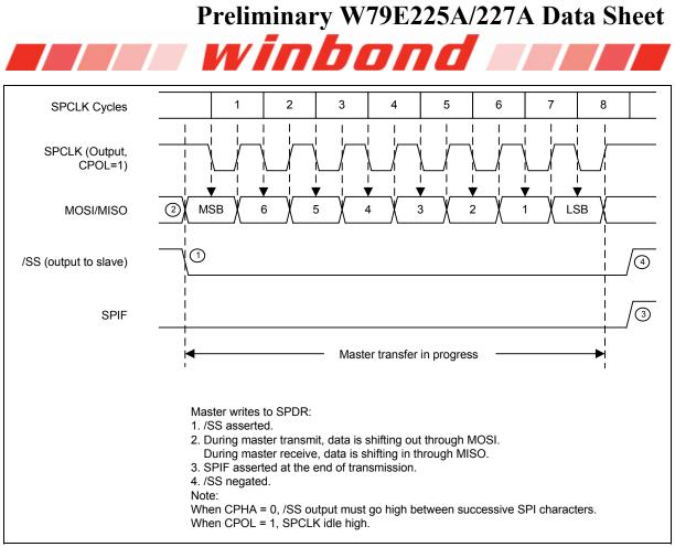
Figure 18-3: Master Mode Transmission (CPOL = 1, CPHA = 0)
