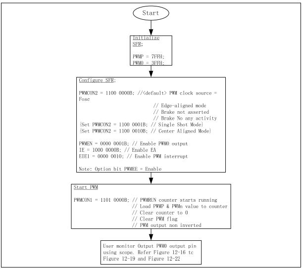
Figure 14-18: Program Flow for Edge-Aligned mode
