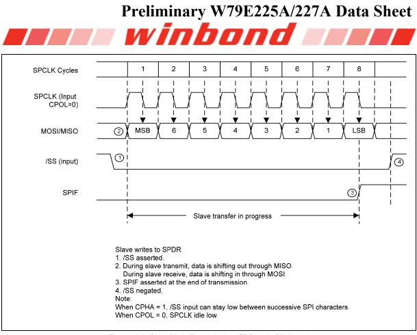
Figure 18-8: Slave Mode Transmission (CPOL = 0, CPHA = 1)
