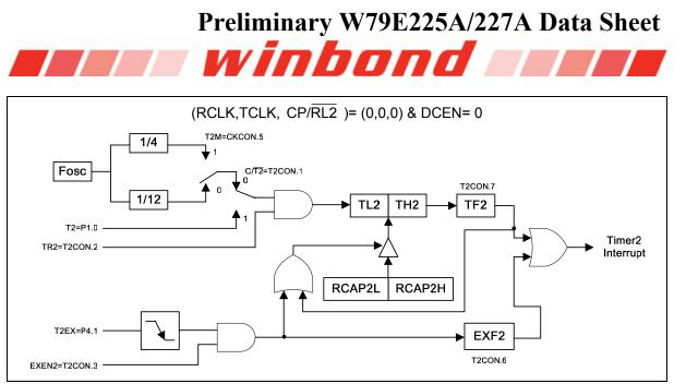
Figure 12-5: 16-Bit Auto-reload Mode, Counting Up
