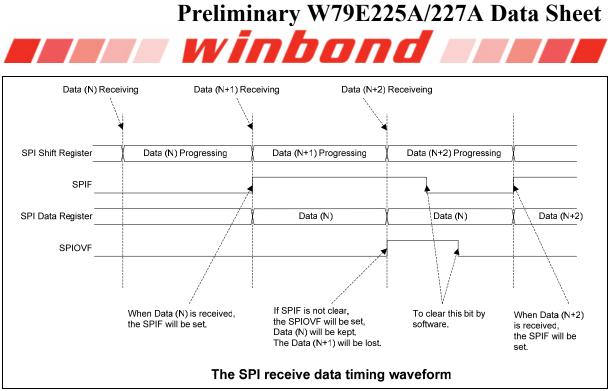
Figure 18-11: SPI Overrun Timing Waveform
