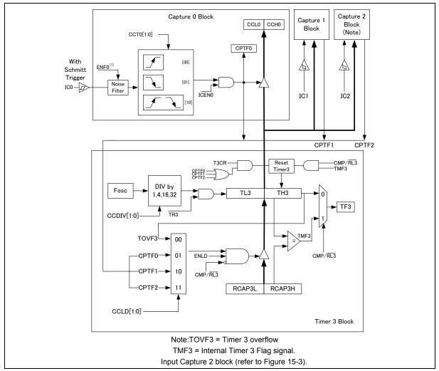
Figure 15-2: Timer3/Capture/Compare/Reload modules
