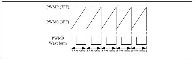
Figure 14-19: PWM0 Edge Aligned Waveform Output
