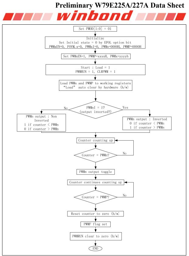
Figure 14-24: Single-Shot Flow Diagram
