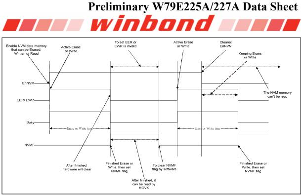
Figure 6-5: NVM data memory control timing
