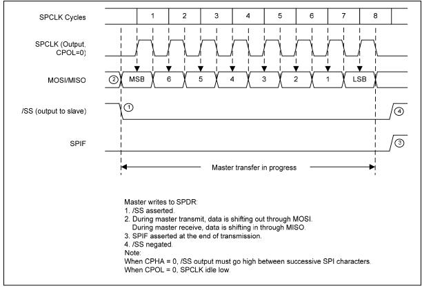
Figure 18-2: Master Mode Transmission (CPOL = 0, CPHA = 0)
