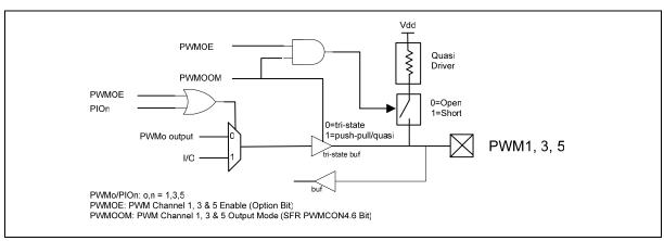
Figure 14-4: PWM1, 3 & 5 I/O pins
