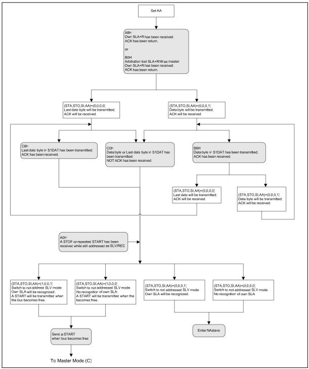
Figure 17-7: Slave Transmitter Mode
