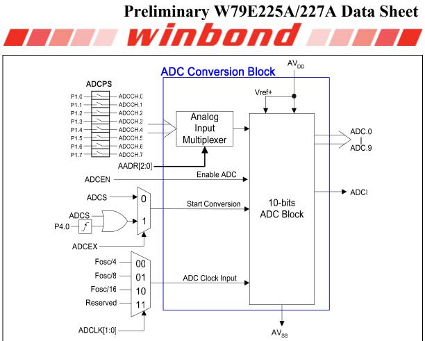
Figure 19-2: ADC Block Diagram
