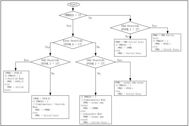
Figure 14-12: Override Flow Diagram
