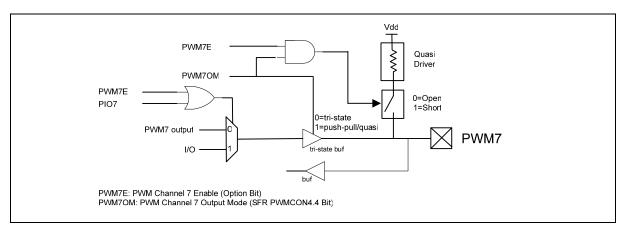
Figure 14-6: PWM7 I/O pin
