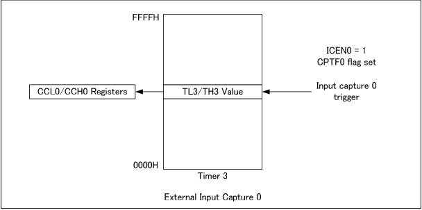
Figure 15-9: Input Capture 0 Triggers
