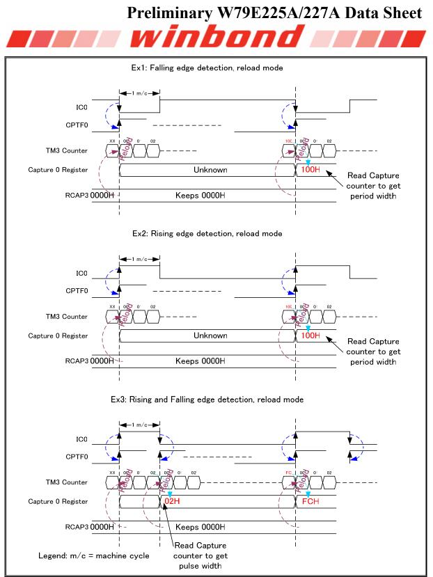
Figure 15-4: Timing diagram for Input Capture
