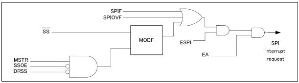
Figure 18-10: SPI interrupt request
