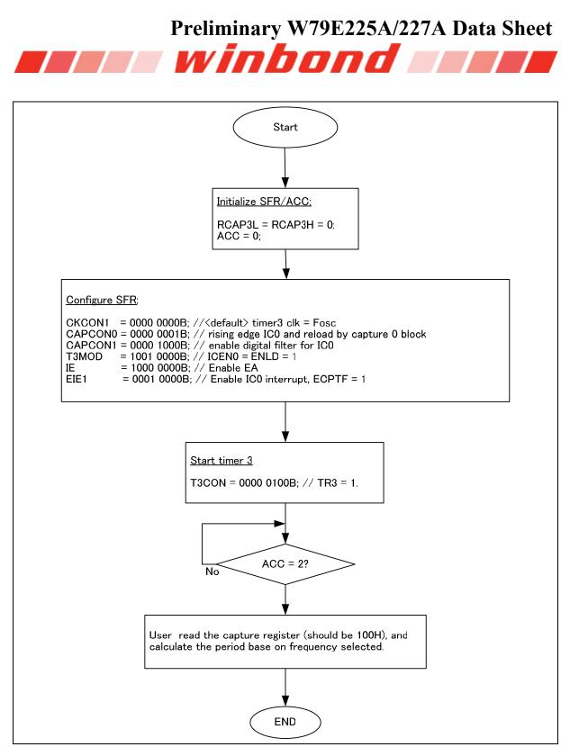
Figure 15-6: Program flow for measurement with IC0 between pulses with rising edge detection (ACC is incremented in interrupt service routine).
