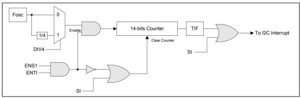
Figure 17-3: I2C Time-out Block Diagram
