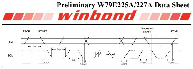
Figure 24-1: I2C Bus Timing
