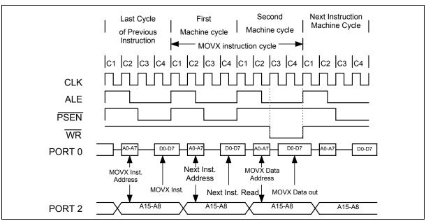
Figure 8-6: Data Memory Write with Stretch Value = 0
