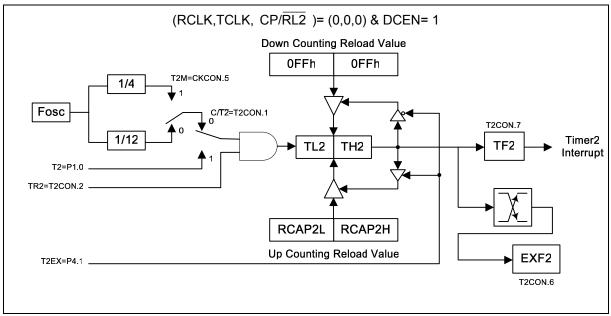
Figure 12-6: 16-Bit Auto-reload Up/Down Counter
