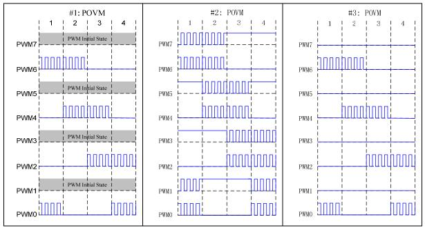
Figure 14-15: Example 2 of Output Override
