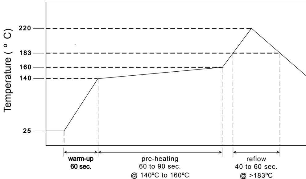
Note: EMXO's are precision subsystems with tolerances measured to  $\pm 0.001$  ppm. The EX-381/5 series has been designed for pick and place reflow soldering. The suggested reflow profile is shown above. The EX-381/5 may be reflowed one time in the non-inverted state. VI recommends waiting at least two hours after reflow before measuring the unit.
