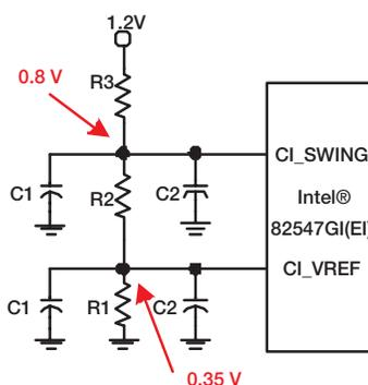
**Figure 2. CSA Port Locally Generated Reference Divider Circuits**
