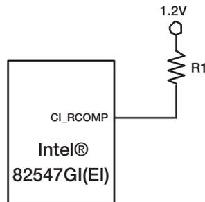
Figure 3. CSA port CI\_RCOMP Circuits
