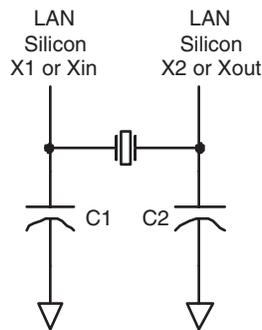
Figure 4. Crystal Circuit
