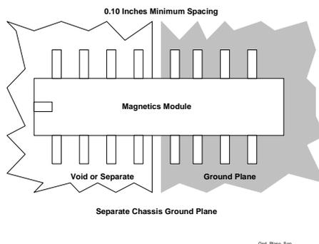
Figure 7. Ground Plane Separation
