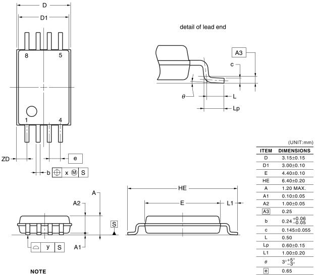
Each lead centerline is located within 0.10mm of its true position at maximum material condition.
