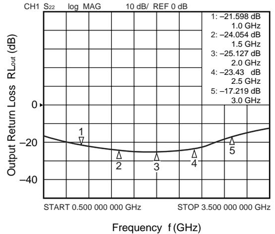
TEST CONDITION:  $T_A = +25^\circ\text{C}$ ,  $f = 1 \text{ GHz}$ ,  $V_{\text{cont1/2}} = 0 \text{ V}$ ,  $3.0 \text{ V}$ , OUT2 side is termination
