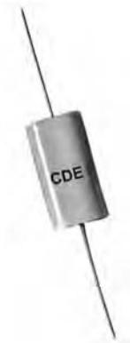
Type 936C flat axial leaded metallized polypropylene capacitors are designed for 20 to 100 kHz switching power supply input filtering, DC blocking and output filter applications where high current, high capacitance and low ESR values are important. Dry sections are sealed with flame retardant outer wrap and epoxy end seals for moisture resistance.
