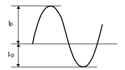
Unbalance rate =  $| l_p - l_{-p} | / l_L \times 100$  (%) Wave-height rate =  $l_p$  (or  $l_{-p}$ ) /  $l_L$
