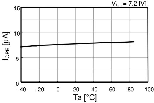
Current consumption vs. temperature in power-down mode
