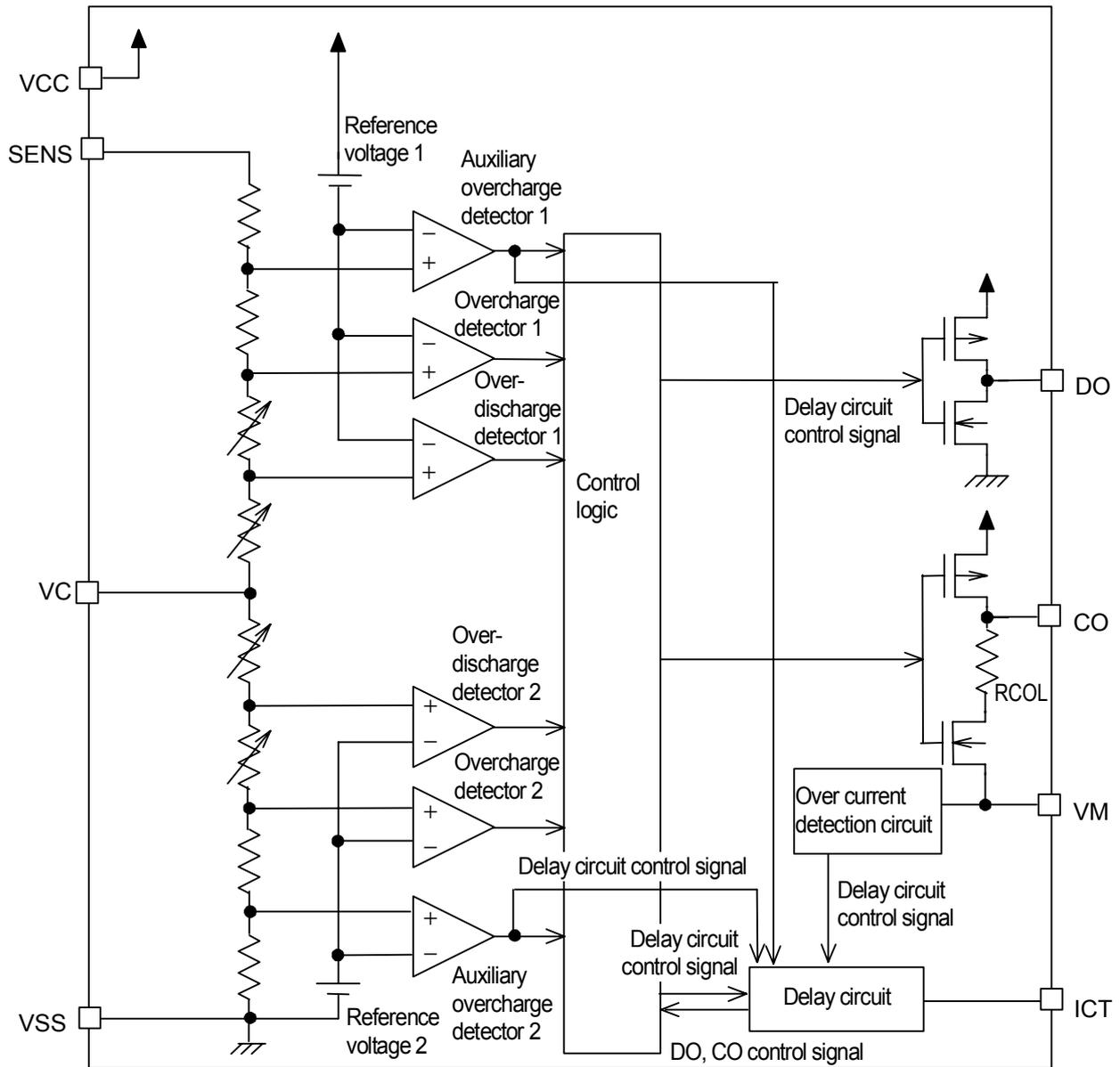
**Remark** Resistor (RCOL) is connected to the Nch transistor although CO pin serves as a CMOS output. For this, impedance becomes high when outputting "L" from CO pin. Refer to the "■ **Electrical Characteristics**" for the impedance value.
