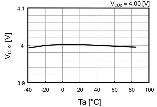
Auxiliary overcharge detection voltage1 vs. temperature
