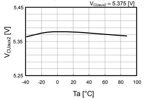
Overdischarge detection voltage1 vs. temperature
