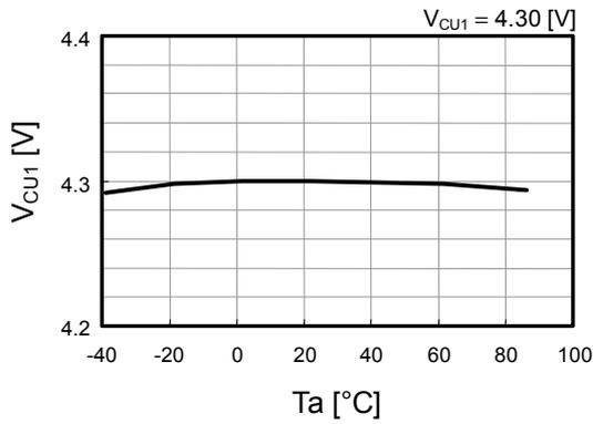
Overcharge detection voltage2 vs. temperature
