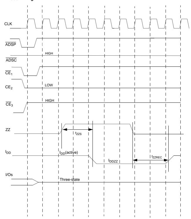
20. Device must be deselected when entering ZZ mode. See Cycle Description table for all possible signal conditions to deselect the device.
