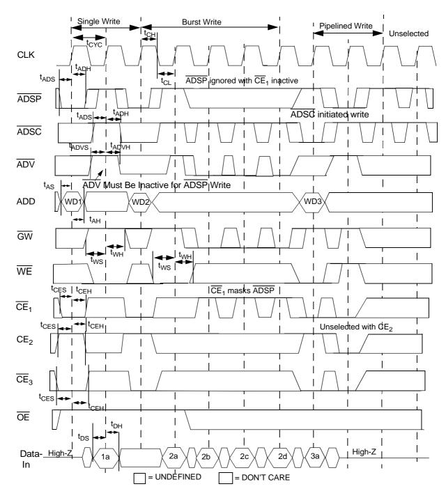
$<sup>\</sup>overline{WE}$  is the combination of  $\overline{BWE}$ ,  $\overline{BW}_{[3:0]}$  and  $\overline{GW}$  to define a write cycle (see Write Cycle Descriptions table). WDx stands for Write Data to Address X.
