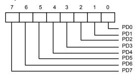
The contents of DB0-DB7 are buffered (non-inverting) and output to ports PD0-PD7 during a write operation. The leading edge of IOW# causes an EPP address write cycle to be performed, and the trailing edge of IOW# latches the data for the duration of the EPP write cycle.
