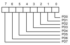
When accesses are made to any EPP data port, the contents of DB0-DB7 are buffered (non-inverting) and output to the ports PD0-PD7 during a write operation. The leading edge of IOW# causes an EPP data write cycle to be performed, and the trailing edge of IOW# latches the data for the duration of the EPP write cycle.
