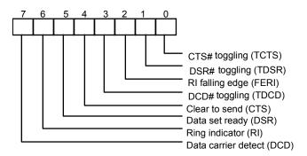
Bit 7: This bit is the opposite of the DCD# input. This bit is equivalent to bit 3 of HCR in loopback mode.
