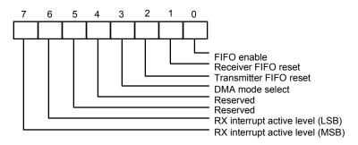
Bit 6, 7: These two bits are used to set the active level for the receiver FIFO interrupt. For example, if the interrupt active level is set as 4 bytes, once there are more than 4 data characters in the receiver FIFO, the interrupt will be activated to notify the CPU to read the data from the FIFO.
