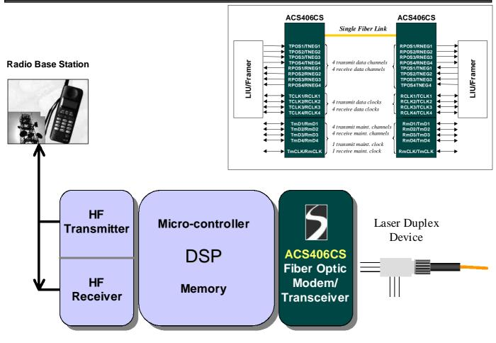
Up to 4 x E1/T1 + maintenance Single fiber link up to 25km
