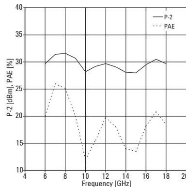
**Figure 3. Typical Output Power (@P-2) and PAE**
