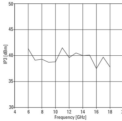
**Figure 5. Typical Output 3<sup>rd</sup> Order Intercept Pt.**
