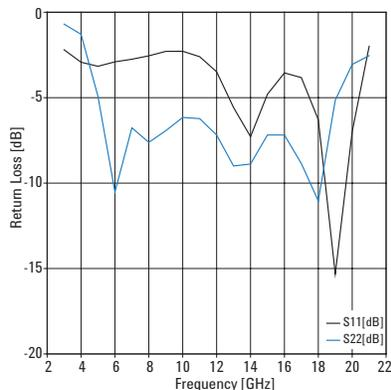
**Figure 2. Typical Return Loss (Input and Output)**
