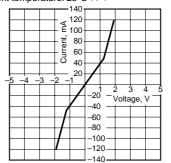
9. Off state leakage current
