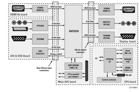
AVC2510 Evaluation system high-level block diagram
