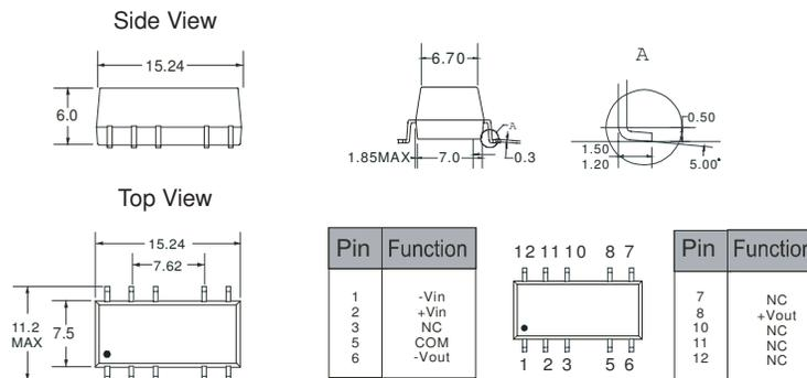
Note: All Pins on a 2.54mm pitch; all pin diameters are 0.50mm; all dimensions in mm.
