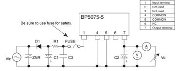
For actual usage, Please kindly evaluate and confirm our part mounted in your product, Especially, Please make sure to confirm whether the load current exceed Max. rated current by using the current probe.
