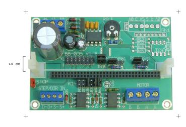
INFO The baseboard BB-035 allows to build a ready to use stepper driver unit using the TMCM-035 driver module. All important signal and power lines are accessible via screw terminals, the step and direction inputs are equipped with opto couplers. The integrated switch-mode regulator provides the required 5V supply voltage for the TMCM-035.
