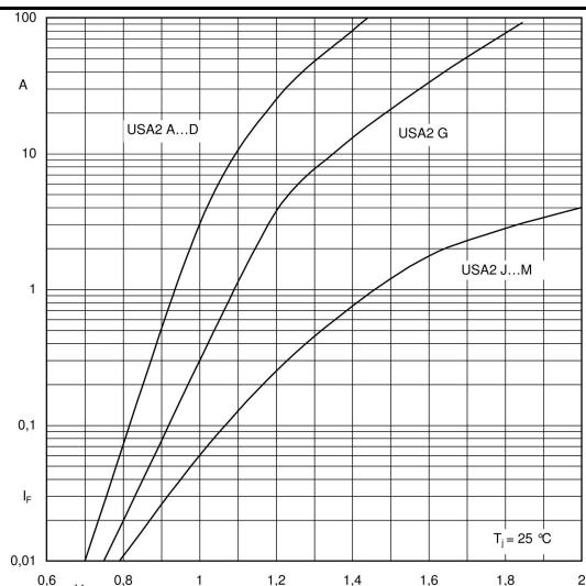
Fig. 1 Forward characteristics (typical values)
