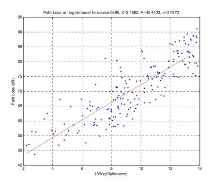
Figure 2: Path loss vs. log distance
