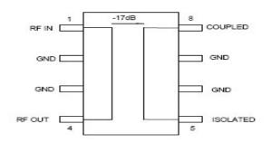
Note: Pins 2, 3, 6 and 7 must be RF and DC grounded.
