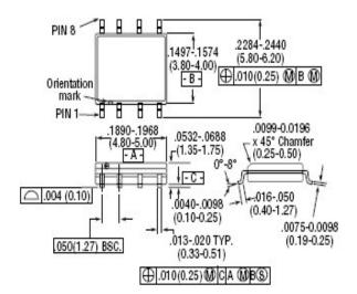
8- Lead SOP outline dimensions Narrow body .150 (All dimensions per JEDEC No. MS-012-AA, Issue C) Dimensions in ( ) are in mm.
