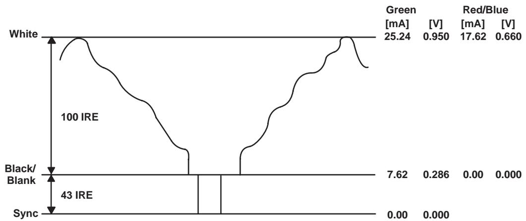
Figure 2-18. Composite Video Output (With 0 IRE, 8-Bit Output)
