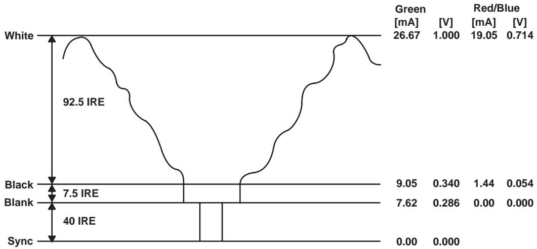
Figure 2-17. Composite Video Output (With 7.5 IRE, 8-Bit Output)
