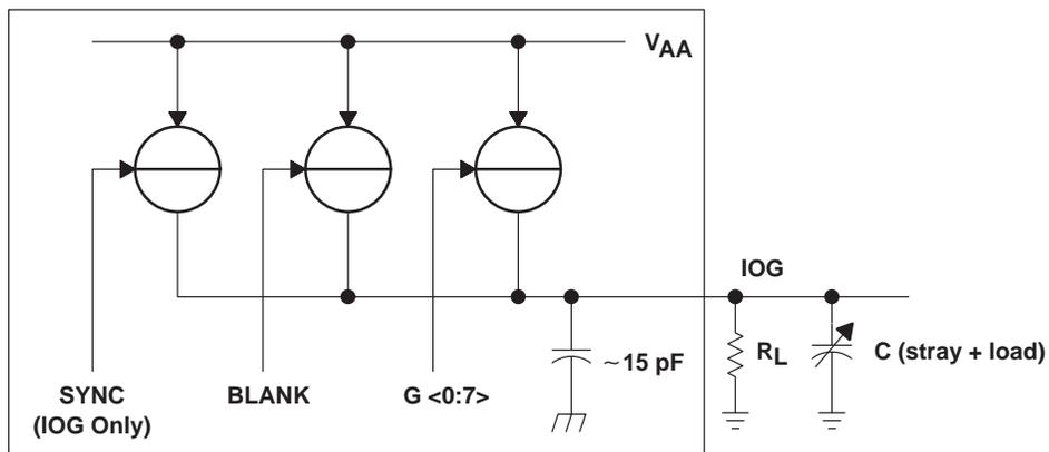
Figure 2–16. Equivalent Circuit of the IOG Current Output
