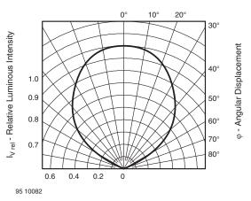
Fig. 2 - Rel. Luminous Intensity vs. Angular Displacement
