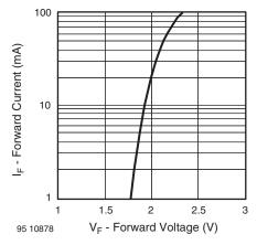
Fig. 3 - Forward Current vs. Forward Voltage
