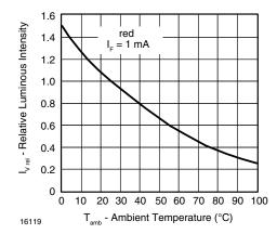
Fig. 5 - Rel. Luminous Intensity vs. Ambient Temperature
