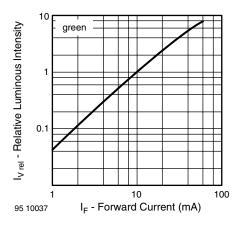
Fig. 16 - Relative Luminous Intensity vs. Forward Current
