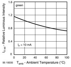
Fig. 14 - Rel. Luminous Intensity vs. Ambient Temperature
