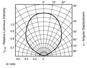
Fig. 2 - Rel. Luminous Intensity vs. Angular Displacement
