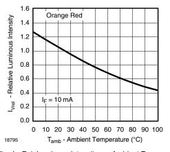
Fig. 4 - Rel. Luminous Intensity vs. Ambient Temperature
