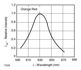
Fig. 7 - Relative Intensity vs. Wavelength
