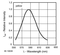
Fig. 12 - Relative Intensity vs. Wavelength
