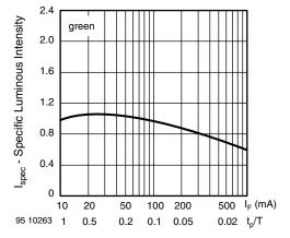
Fig. 15 - Specific Luminous Intensity vs. Forward Current
