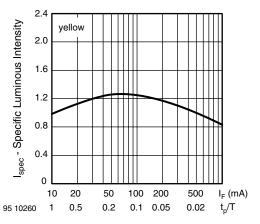
Fig. 10 - Rel. Lumin. Intensity vs. Forw. Current/Duty Cycle
