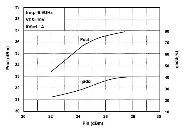
Output Power(Pout) vs. Input Power(Pin)
