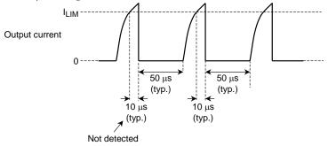
The target specification for the overcurrent limiter value (overcurrent threshold) is 2.5 A (typ.), and varies in a range from approximately 1.5 A to 3.5 A.
