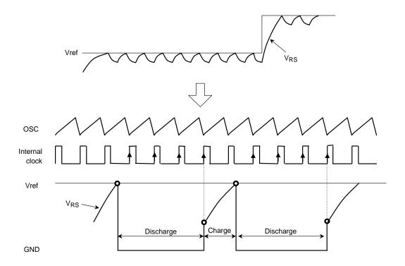
2) Transition from charge mode to discharge mode If VRS > Vref after four clock signals in charge mode, the IC again enters discharge mode. After a further four clock signals in discharge mode, VRS is compared with Vref. If VRS < Vref, the IC operates in charge mode until VRS reaches Vref.
