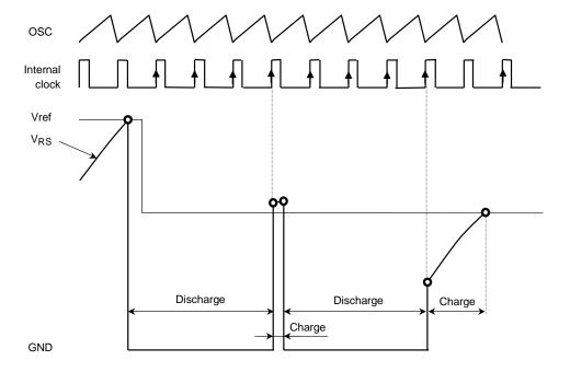
(3) Transition from discharge mode to charge mode
