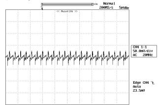
**Figure 14:** Output voltage ripple at nominal input voltage and rated load current (Io=5A)(50 mV/div, 5us/div).Load capacitance: 1μF ceramic capacitor and 10μF tantalum capacitor. Bandwidth: 20 MHz. Scope measurements should be made using a BNC cable (length shorter than 20 inches). Position the load between 51 mm to 76 mm (2 inches to 3 inches) from the module
