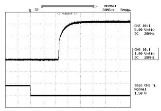
**Figure 4:** (For negative remote on/off logic) Turn-on transient at full rated load current (5 ms/div). Vin=48V. Top Trace: Vout, 1V/div; Bottom Trace: ON/OFF input, 5V/div.
