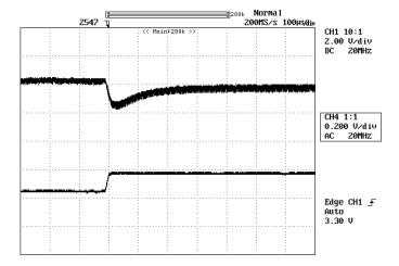
**Figure 9:** Output voltage response to step-change in load current (50%-75% of lo, max; di/dt = 0.1A/ $\mu$ s). Load cap:  $10\mu$ F tantalum capacitor and  $1\mu$ F ceramic capacitor. Top Trace: Vout (200mV/div, 100us/div), Bottom Trace: lout (2A/div). Scope measurement should be made using a BNC cable (length shorter than 20 inches). Position the load between 51 mm to 76 mm (2 inches to 3 inches) from the module.
