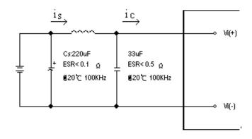
**Figure 10:** Test set-up diagram showing measurement points for Input Terminal Ripple Current and Input Reflected Ripple Current. Note: Measured input reflected-ripple current with a simulated source Inductance ( $L_{TEST}$ ) of 12  $\mu$ H. Capacitor Cs offset possible battery impedance. Measure current as shown below.
