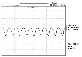
**Figure 11:** Input Terminal Ripple Current, i<sub>c</sub>, at full rated output current and nominal input voltage with 12μH source impedance and 33μF electrolytic capacitor (100mA/div, 2us/div)
