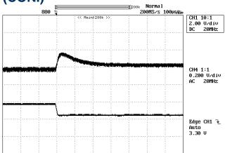
Figure 8: Output voltage response to step-change in load current (75%-50% of lo, max; di/dt = 0.1A/μs). Load cap: 10μF tantalum capacitor and 1μF ceramic capacitor. Top Trace: Vout (200mV/div, 100us/div), Bottom Trace: lout (2A/div). Scope measurement should be made using a BNC cable (length shorter than 20 inches). Position the load between 51 mm to 76 mm (2 inches to 3 inches) from the module.
