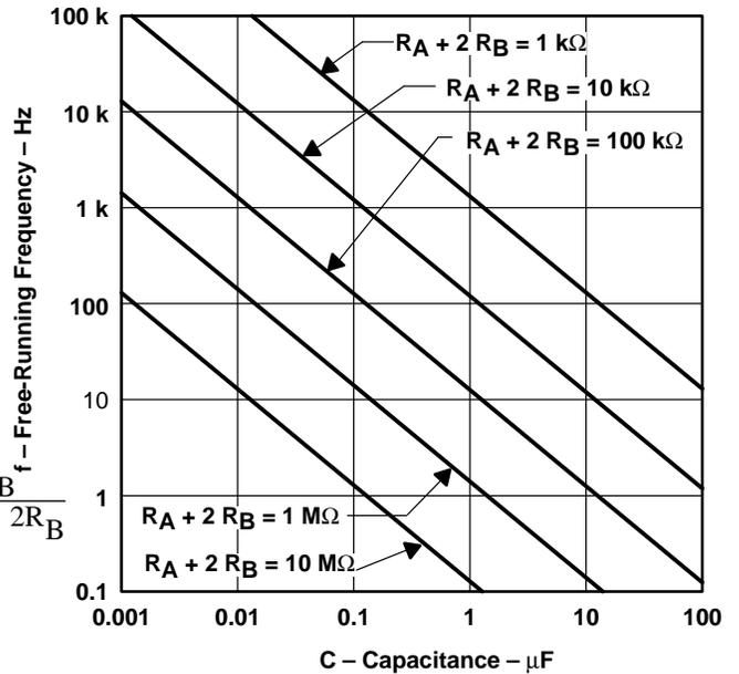
Figure 14. Free-Running Frequency
