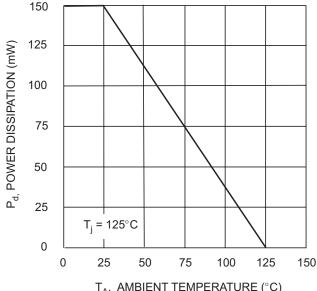
T<sub>A</sub>, AMBIENT TEMPERATURE (°C) Fig. 1 Derating Curve
