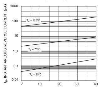
V<sub>R</sub>, INSTANTANEOUS REVERSE VOLTAGE (V) Fig. 3 Typical Reverse Characteristics
