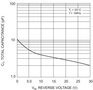
Fig. 4 Total Capacitance vs. Reverse Voltage
