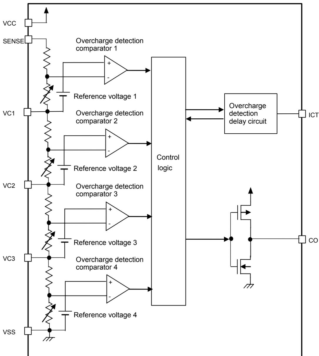
**Remark** In the case of Nch open-drain output, only the Nch transistor will be connected to the CO pin. In the case of Pch open-drain output, only the Pch transistor will be connected to the CO pin.
