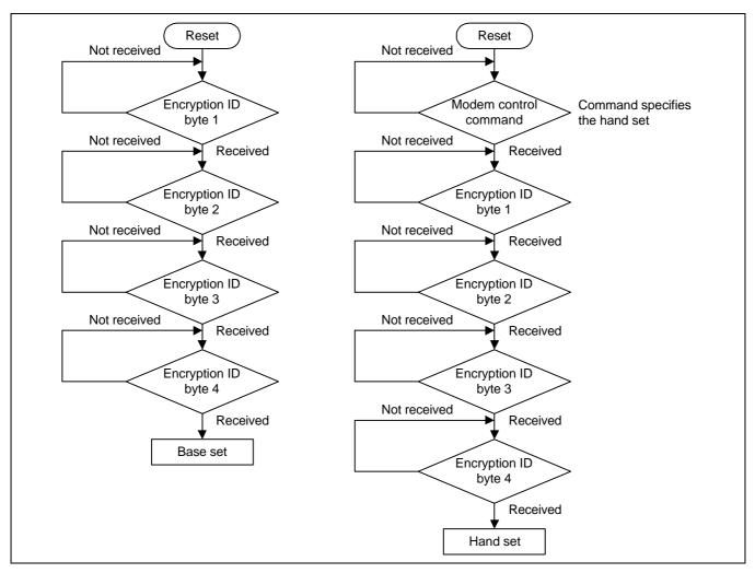
After specifying the hand or base set and encryption ID, the host can operate the S5T8610 in other modes by sending the modem control command specifying the corresponding mode.
