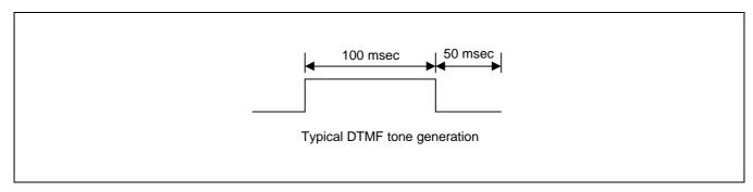
The single tone and continuous tone can be generated using the DTMF control command. The commands and tables related to DTMF generation is shown in the Command Set section.
