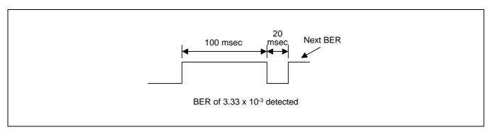
For 24kbps ADPCM, this pin produces high for 20msec when jamming is detected. After producing high, the BER pin produces low for 20msec before detecting the next jamming. Jamming detection is not necessary for 16kbps ADPCM, since BER can be used for detecting jamming.
