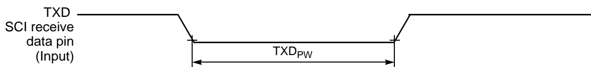
Figure 10-17 TXD Pulse Width
