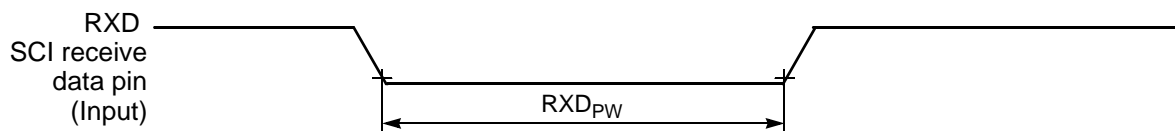
Figure 10-16 RXD Pulse Width
