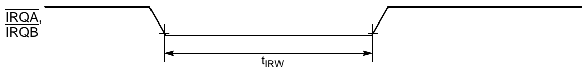
Figure 10-6 External Interrupt Timing (Negative Edge-Sensitive)
