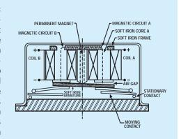
field, it is necessary to apply the correct polarity to the relay coils as indicated on the relay schematic.
