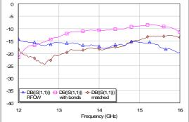
Once bonded the return losses are still at a reasonable level. They can be improved with simple compensation networks. The figures also show the effect of this bondwire compensation network (brown diamonds). The networks are shown at the end of this section.
