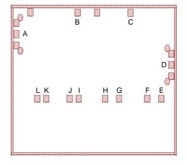
Note: Co-ordinates are referenced from the bottom left hand corner of the die to the centre of bond pad opening. Pads without identifiers are ground connections used in wafer testing.
