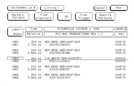
The above display data using the PCI Inverse Assembly software without the PCI PC Mapper functionality is shown as follows.
