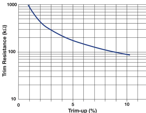
$$R_{\text{TRIM-UP}} = \left\{ \frac{V_o (100+\Delta\%)}{1.225\Delta\%} - \frac{(100+2\Delta\%)}{\Delta\%} \right\} 5.11\text{k}\Omega$$
