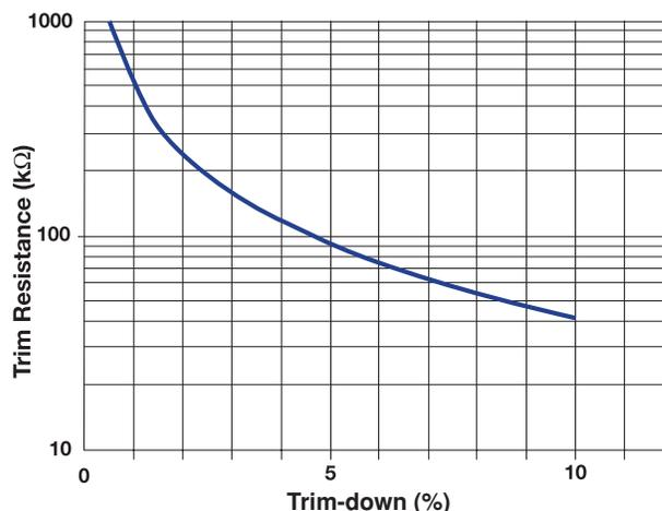
$$R_{\text{TRIM-DOWN}} = \left\{ \frac{100}{\Delta\%} - 2 \right\} 5.11\text{k}\Omega$$
