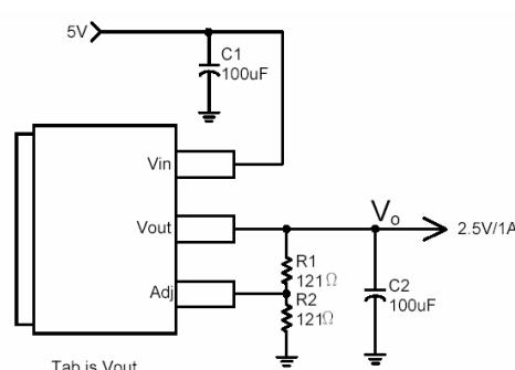
Note:  $V_o = V_{REF} * \left(1 + \frac{R_2}{R_1}\right)$
