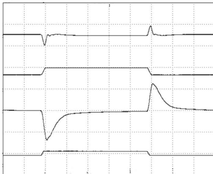
Figure 12: Output voltage response to step-change in load current lout2 and lout1 (75%-50%-75% of I_o , max; di/dt = 0.1A/\mu s ). Load cap: 10\mu F , tantalum capacitor and 1\mu F ceramic capacitor. Ch1=Vout1 (50mV/div), Ch2=lout1 (10A/div), Ch3=Vout2 (100mV/div), Ch4=lout2 (10A/div) Scope measurement should be made using a BNC cable (length shorter than 20 inches). Position the load between 51 mm to 76 mm (2 inches to 3 inches) from the module.
