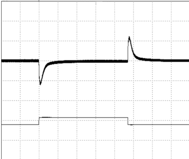
Figure 13: Output voltage response to step-change in load current lout2 (75%-50%-75% of I_o , max; di/dt = 2.5A/\mu s ) at lout1=0. Load cap: 470 \mu F , 35m \Omega ESR solid electrolytic capacitor and 1 \mu F ceramic capacitor. Ch1=Vout2 (50mV/div), Ch2=lout2 (5A/div), Scope measurement should be made using a BNC cable (length shorter than 20 inches). Position the load between 51 mm to 76 mm (2 inches to 3 inches) from the module.
