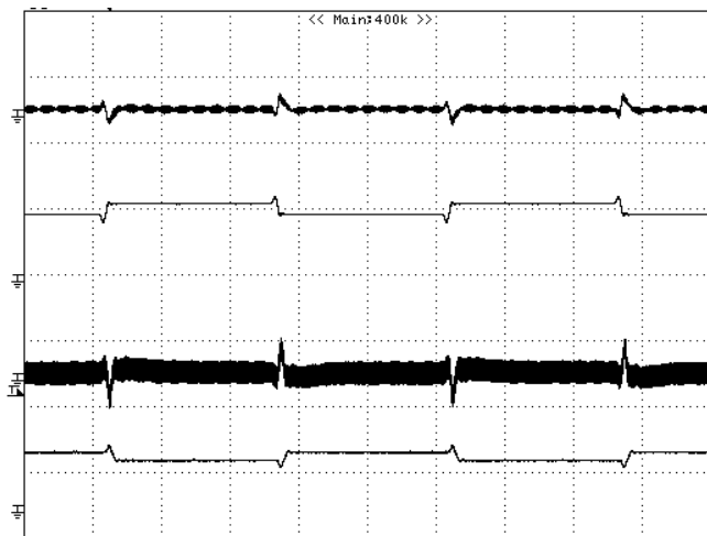
Figure 15: Output voltage response to step-change in load current lout2 and lout1 (75%-50%-75% of I_o , max; di/dt = 2.5A/\mu s ). Load cap: 470 \mu F , 35m \Omega ESR solid electrolytic capacitor and 1 \mu F ceramic capacitor. Ch1=Vout1 (100mV/div), Ch2=lout1 (5A/div), Ch3=Vout2 (100mV/div), Ch4=lout2 (5A/div) Scope measurement should be made using a BNC cable (length shorter than 20 inches). Position the load between 51 mm to 76 mm (2 inches to 3 inches) from the module.
