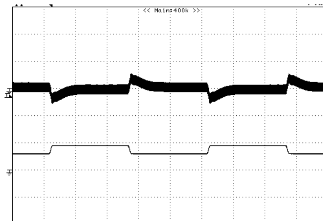
Figure 10: Output voltage response to step-change in load current lout2 (75%-50%-75% of I_o , max; di/dt = 0.1A/\mu s ) at lout1=0A. Load cap: 10\mu F , tantalum capacitor and 1\mu F ceramic capacitor. Ch1=Vout2 (100mV/div), Ch2=lout2 (5A/div), Scope measurement should be made using a BNC cable (length shorter than 20 inches). Position the load between 51 mm to 76 mm (2 inches to 3 inches) from the module.
